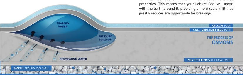
**66** Resin is the largest ingredient in a fibreglass pool shell. Approximately 70% of the pool shell is made from resin. The esters in resin are susceptible to breaking down when exposed to water. ??
